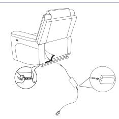
Safety Note: Transformer and cables are not to be placed under or within the recliner structure.
